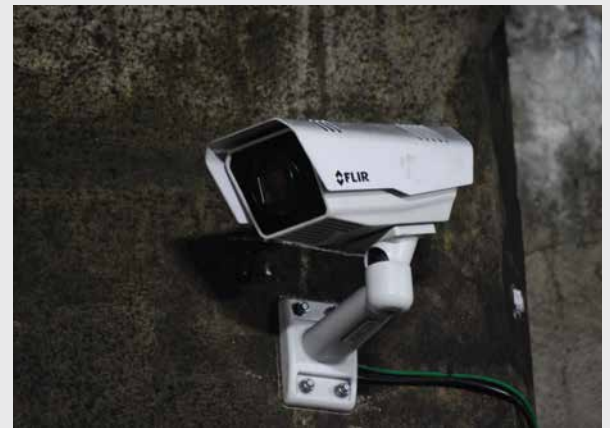
FLIR ITS-Series Rail. FLIR cameras ensure 24/7 detection on tracks or in tunnels and do not need any illumination to operate.
