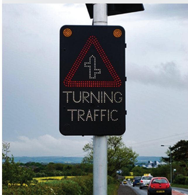
Upon detection by the FLIR TrafiOne, the electronic warning signs are activated.
