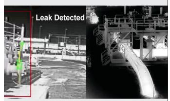
The combination of visual and thermal sensors is an efficient way to monitor the safety of above-line piping facilities.
