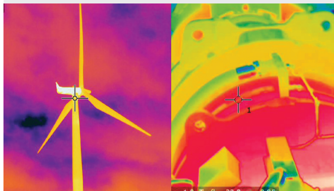
Thermal imaging can be used to detect both electrical and mechanical issues
