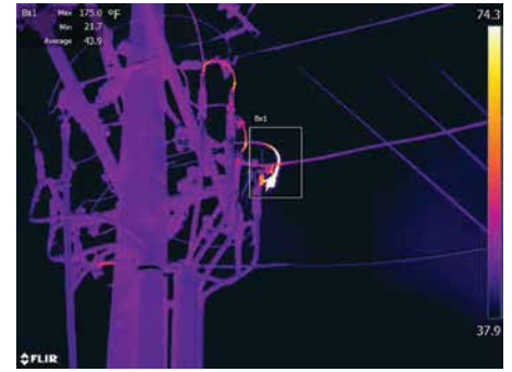
A failing hot tap on the connection between an overhead to underground power line on a riser structure at PUD 3's Union River Substation needed to be repaired quickly to avoid an outage that would have affected about 1,000 customers.
