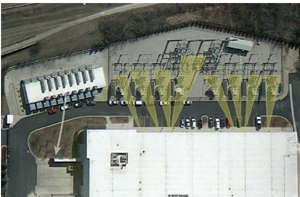
A large Midwestern data center with its own electric substation increased its security level by increasing the thermographic sampling from four times per year to more than 26,000 times per year.
