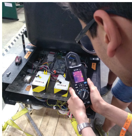
Through IGM, the CM275 provides a reliable way to identify hot spots and overloaded circuits.
