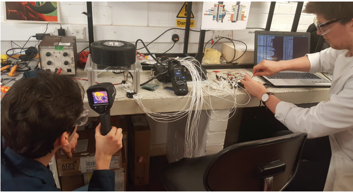
Thermal imaging cameras offer the HYPED team a safer, contactless way to inspect battery packs and electronics.
