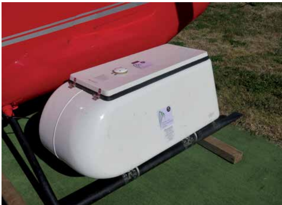
The imaging platform consists of a fully STC certified phenoAIR™ that can be fitted to any R44 helicopter.
