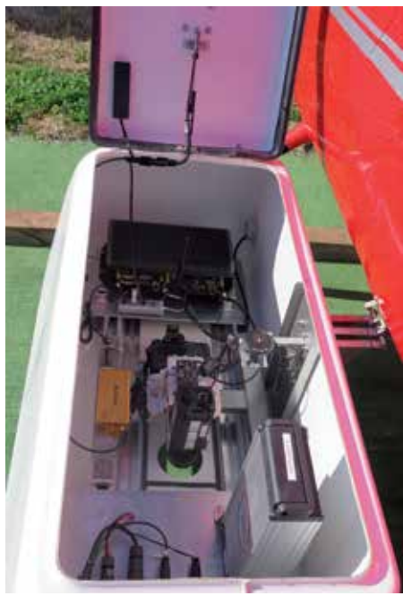
The pod carries an advanced imaging payload consisting of a high resolution FLIR SC645 Infrared camera and 30MP RGB camera, with a fully integrated IMU and GPS.
