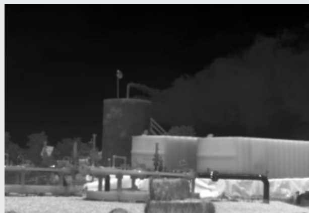
OGI cameras provide detection from a safe distance, displaying gas leaks as visible clouds of smoke. This can be shown in color or black and white as shown above.
