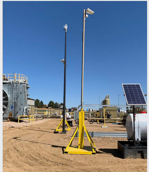
The FLIR G300a cameras were placed on pan-tilt units, allowing maintenance operators to surveil the whole property with optical gas imaging technology.
