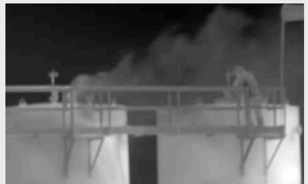
Opening the thief hatch is a large emitter of volatile organic compounds (VOC), which damage the environment and raise safety concerns for workers.
