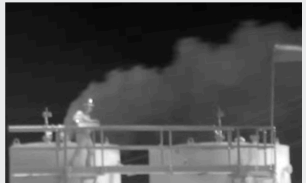
The FLIR G300a cameras were placed on pan-tilt units, allowing maintenance operators to surveil the whole property with optical gas imaging technology.
