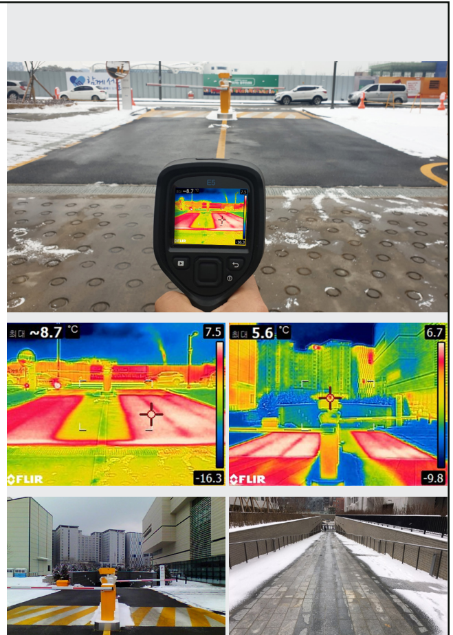
Visual image (above) and thermal image of a road with an embedded snow-melting system.
