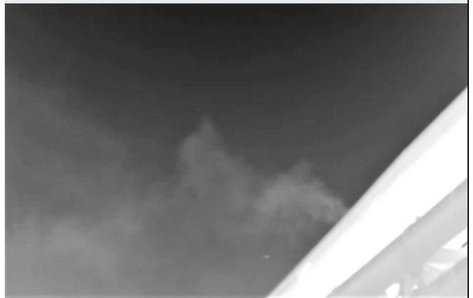
Image of a carbon monoxide (CO) leak in normal mode from a blast furnace during normal operation
