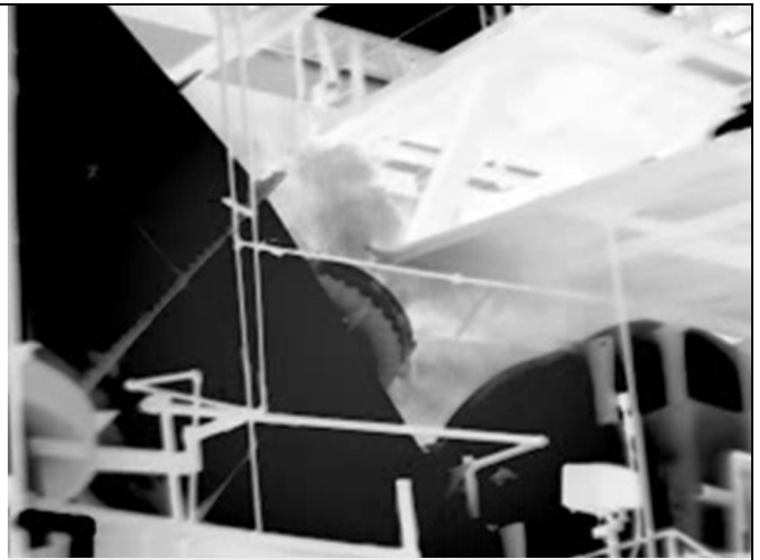
CO leak from a bleeder valve detected with the FLIR GF346 camera
