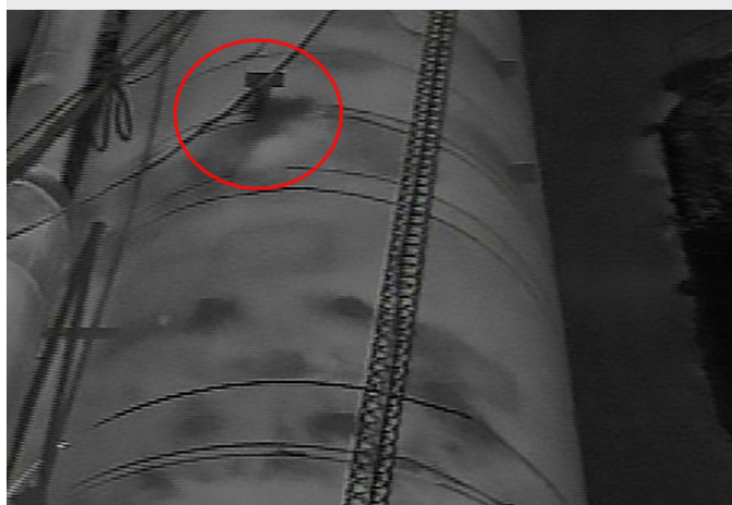
CO pipeline leak identified with a FLIR GF346 optical gas imaging camera
