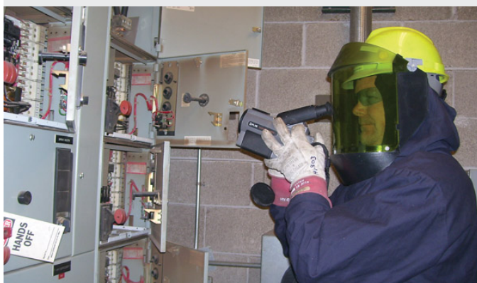
Infrared scanning is applicable on all electrical assets including motor control centers, but typically requires extensive PPE if done “open panel”
