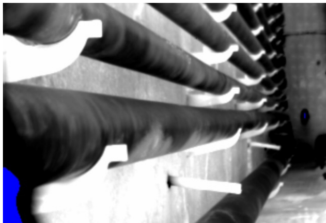
Fig. 3. Areas of the tubes suffering from internal coking show soft edges and a “ghostly glow” in the thermal image, indicating actual hotter tube areas that might be overheating.
