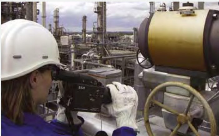
Examining potential leak paths
